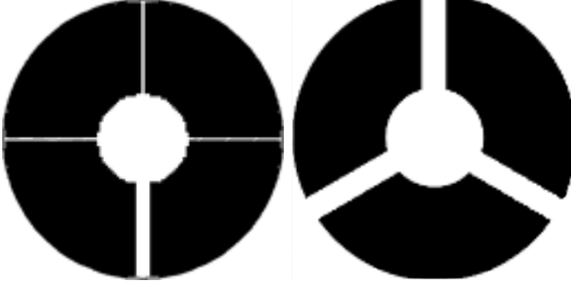
Figure 3.3: Telescope pupil examples: Negative of the pupil footprints from the Sunrise III (left, Korpi-Lagg et al. 2025) and HINODE SOT (right, Kosugi et al. 2007) telescopes in discrete pixel space b : \mathcal{V} \subset \mathbb{R}^2 \rightarrow \{0, 1\} .
